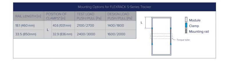
Distance between outer edge of module and middle of the clamp.
