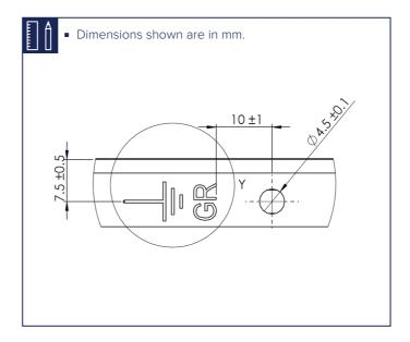
Grounding or bonding should be carried out with Zn-based coated connecting elements to avoid the galvanic coupling effect.
