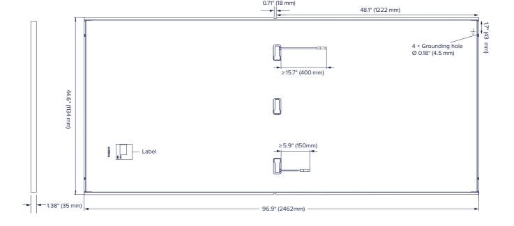
Fig. 1: External dimensions and components for Q.PEAK DUO RSF XL-G11S.3/BFG
