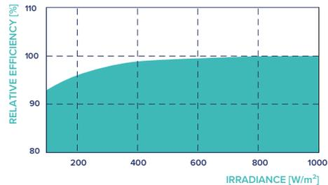
Typical module performance under low irradiance conditions in comparison to STC conditions (25°C, 1000 W/m<sup>2</sup>).
