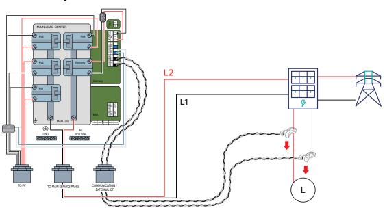
Due to bi-directional energy flow, consumption metering has specific polarity to define whether the power is importing or exporting. The consumption CTs should be installed appropriately according to the direction indication label attached on the edge of the clamp CTs. The red arrow represents the marking on the consumption CTs. Although both the Grid (PV + Load) side and the Load side are acceptable, we recommend using the Grid (PV + Load) side.
