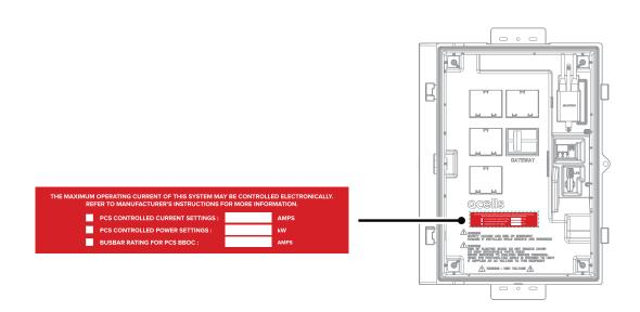
Q.HOME COMBINER also provides PCS labels for current transformers. Apply these labels to the current transformers that enable the PCS modes. Align the white line on the label with the wires near the conductor of the current transformer, then fold the left side and attach it.
