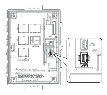
3 Insert the Wi-Fi dongle into the USB port.
