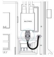
Restore the deadfront cover and plug the USB cable on the USB port marked as 'LTE' on the deadfront.
