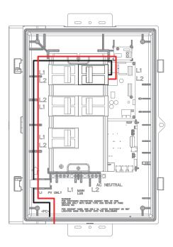
6 Connect L1 and L2 (usually one black and one red) from each AC branch circuit to the circuit breaker(s).
