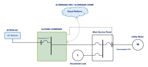
The Solar Configuration is comprised of an AC module (microinverter integrated solar module) and combiner, which consolidates solar modules into a single output. This configuration is ideal for the homeowner wishing to minimize their utility bill and carbon footprint without having a backup power source. Installers can easily upgrade the system in the future by adding energy storage.
