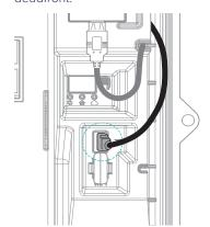
2 Attach the fixture with two screws (M4 - 6 mm) at the cellular attachment part of the deadfront.
