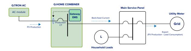
Figure 3. Consumption CTs not installed
