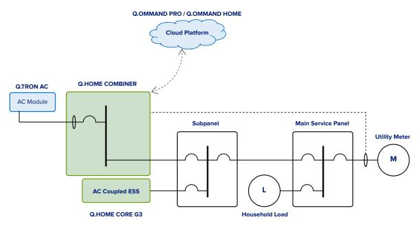
The Grid Support Configuration is comprised of an AC module (microinverter integrated solar module), AC combiner and battery system. This configuration is ideal for the homeowner wishing to save excess power and utilize it when power from grid is expensive.
