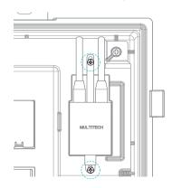
4 Use the slot on the back of the deadfront to arrange the cable.
