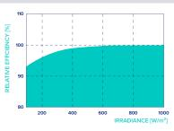
Typical module performance under low irradiance conditions in comparison to STC conditions (25 °C,  $1000 \, \text{W/m}^2$ ).
